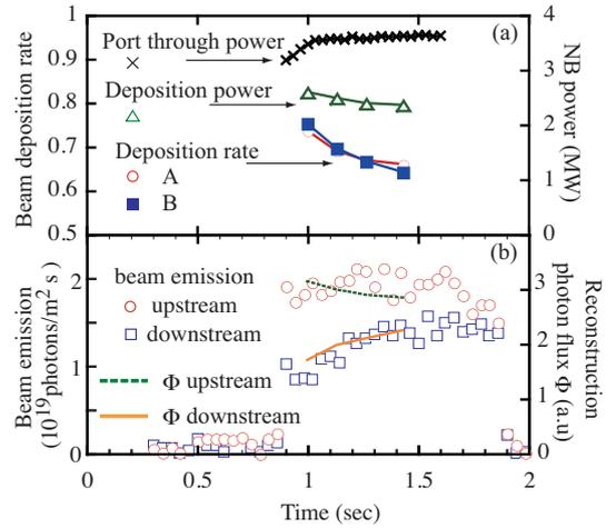
Fig. 5 Time evolution of the beam deposition power obtained by the beam attenuation rate and the port through power (a). Photon fluxes of the beam emission at upstream position (dotted line) and downstream position (bold line) reconstructed by the beam attenuation rate and the beam emission coefficient are plotted on the measured beam emission intensities (b).
