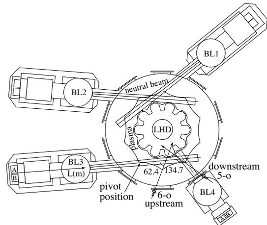
Fig. 1 Schematic top view of the LHD and neutral beam injectors. Two optical sight lines to measure hydrogen beam emission light is set at the upstream position and the downstream position.
