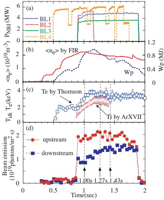
Fig. 2 Time evolutions of injected neutral beam powers (a), the line averaged  $n_e$  and stored energy  $W_p$  (b), the  $T_i$  and  $T_e$  (c), and the beam emission intensities at upstream and downstream (d).
