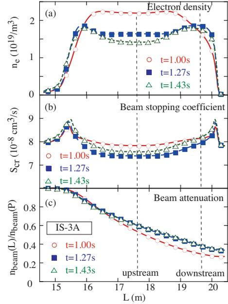
Fig. 4 Along the beam injection axis of IS-3A, the distribution of  $n_e$  (a), and the beam emission coefficient obtained by ADAS data (b), and the neutral beam attenuation factor (c) with the peak density distribution (circle marks) or the hollow density distribution (square marks and triangle marks). Dotted lines are the observed positions at the upstream and the downstream
