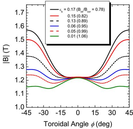
Fig.2 Variation of the magnetic field strength along the magnetic axis for several  $\varepsilon_b$  configurations.
