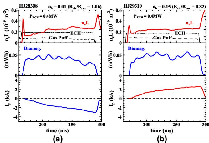
Fig.7 Time traces of electron density, diamagnetic signal and non-inductive toroidal plasma current for (a) the low- and (b) high- $\varepsilon_b$  configurations in the ECCD experiment. ( $\omega_0/\omega \approx 0.49$ )
