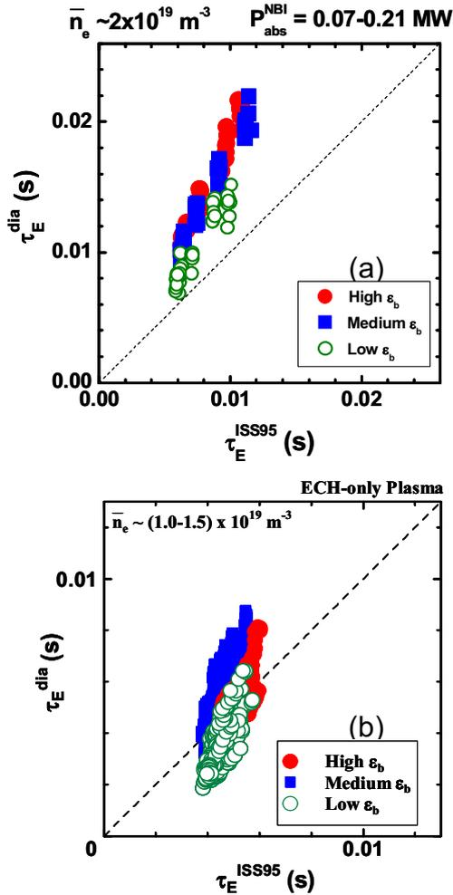
Fig.5 Comparison between  $\tau_E^{\text{dia}}$  and  $\tau_E^{\text{ISS95}}$  for (a) NBI-only plasmas and (b) ECH-only plasma.
