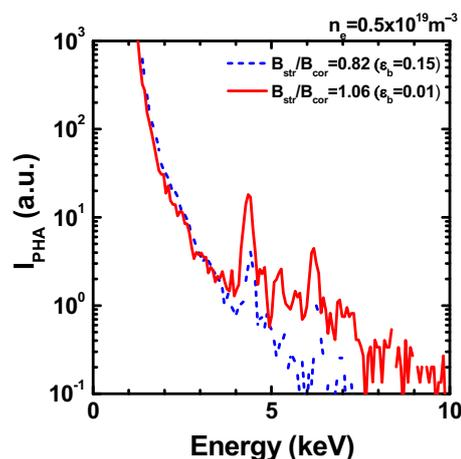
Fig.8 SX spectra for ripple-top ( $B_{\text{str}}/B_{\text{cor}} = 0.82$ ) and ripple-bottom ( $B_{\text{str}}/B_{\text{cor}} = 1.06$ ) heating cases.
