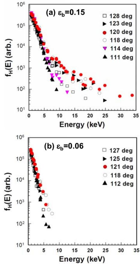
Fig.3 Energy spectra of minority ions (H) for various pitch angles (a) in the high bumpy configuration and (b) in the medium bumpy configurations.
