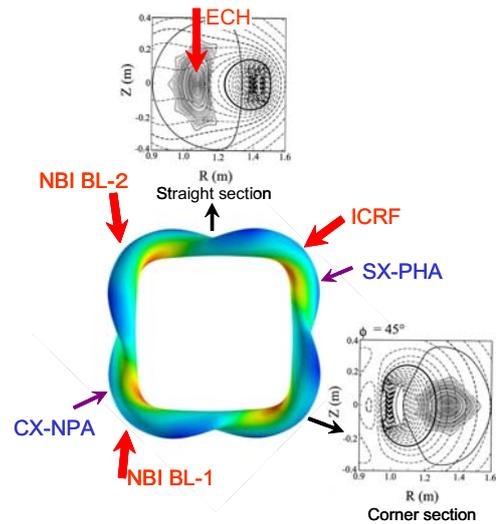
Fig.1 Top view of the magnetic-surface shape (at  $\rho = 0.9$ ) for the standard configuration. The nested magnetic surfaces and the mod-B surfaces at two poloidal sections (straight and corner sections) are also illustrated.
