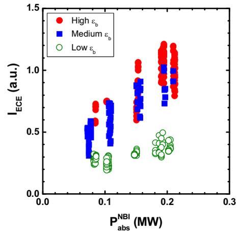
Fig.6 ECE intensity as a function of  $P_{\text{abs}}^{\text{NBI}}$  in high-, medium- and low- $\epsilon_b$  configurations.
