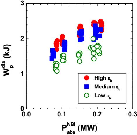
Fig.4 Stored energy obtained in high-, medium- and low- $\epsilon_b$  configurations as a function of absorbed beam power for NBI-only plasmas.
