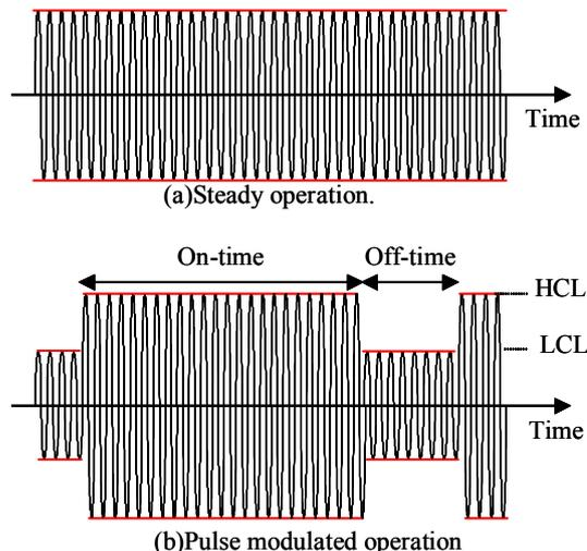
Fig. 1. Pulse modulated coil current
