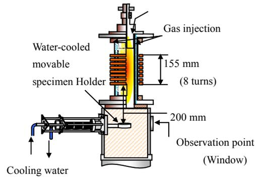
Fig. 2 Schematic diagram of the plasma torch and the observation position
