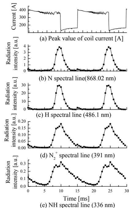
Fig. 4 Time evolution in (a) Peak value of coil current, radiation intensity of (b) N, (c) H, (d) N<sub>2</sub><sup>+</sup>, and (e)NH spectral line
