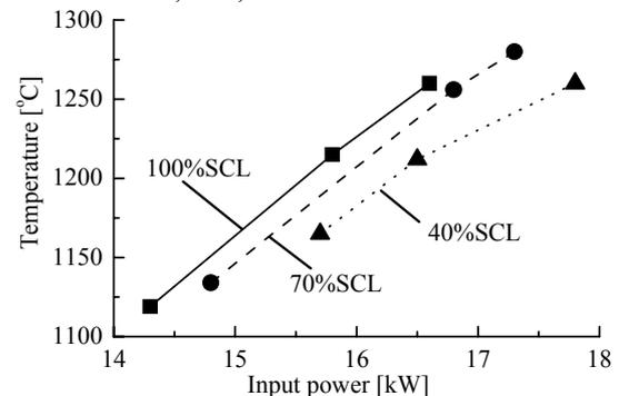
Fig. 7 Dependence of surface temperature of Ti sample on input power.
