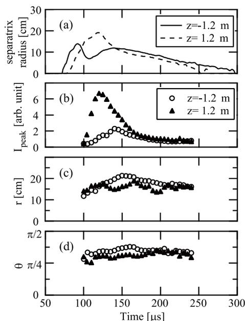
Fig.5 (a) Time evolution of separatrix radius at the axial sections of two tomography devices. (b) Temporal evolution of the peak intensity of the reconstructed light emissivity profiles. (c)-(d) Time evolution of the location of the peak of the reconstructed light emissivity profiles in the polar coordinate.
