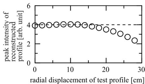
Fig.6 The peak intensity of reconstructed profile as a function of radial displacement of Gaussian-type test profile. The dashed line corresponds to the peak intensity of the test profile.
