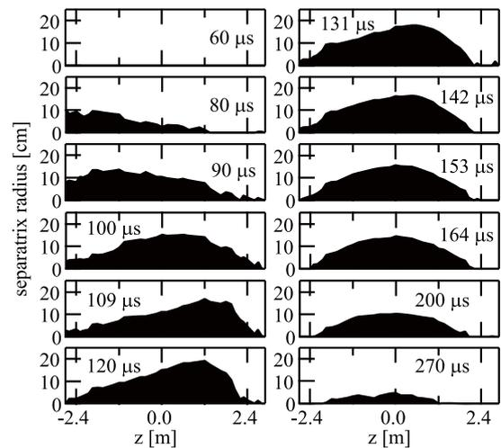
Fig.2 Temporal evolution of the axial profile of separatrix radius of a translated FRC plasma.
