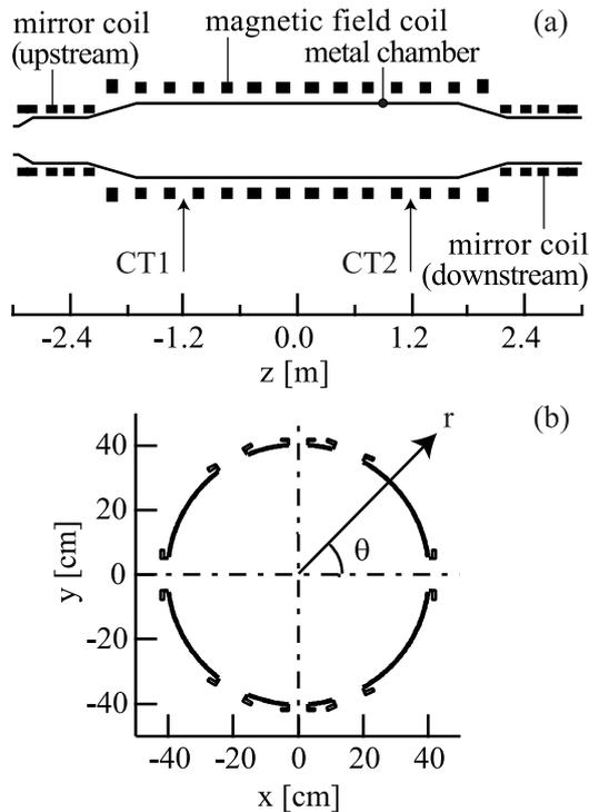
Fig.1 (a) Schematic drawing of the confinement region of the FIX machine. Two computer tomography devices (CT1 and CT2) are located at the axial sections of  $z = -1.2$  and  $1.2$  m. (b) Cross-sectional view of the metal chamber of the central section.
