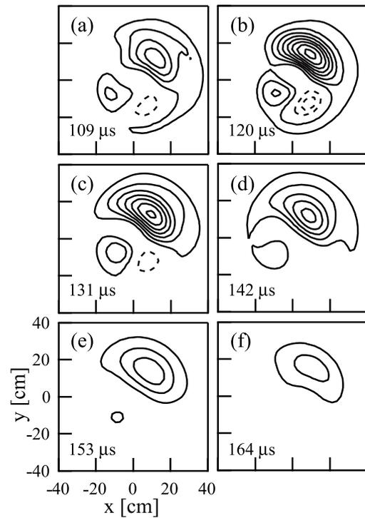
Fig.4 Reconstructed light emissivity profiles of the translated FRC plasma at the axial section of  $z = 1.2$  m in linear-scale intensity. Dashed contours correspond to negative components.
