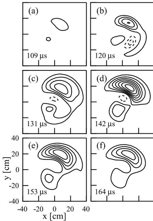
Fig.3 Reconstructed light emissivity profiles of the translated FRC plasma at the axial section of  $z = -1.2$  m in linear-scale intensity. Dashed contours correspond to negative components.
