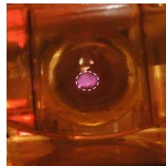
Fig. 4 Photograph of micro-barrier discharges.
