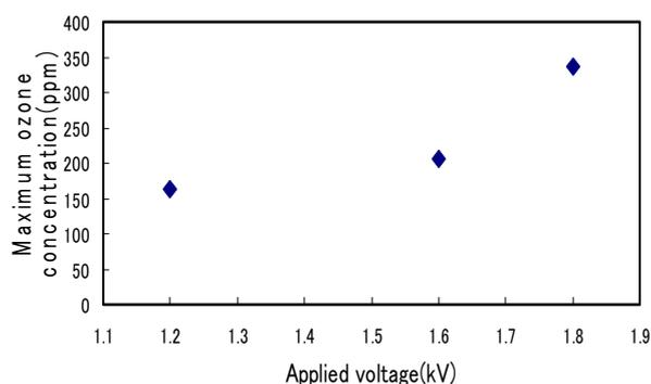
Fig. 10 Ozone concentration after quitting ac voltage and setting the gas pressure at 122kPa.
