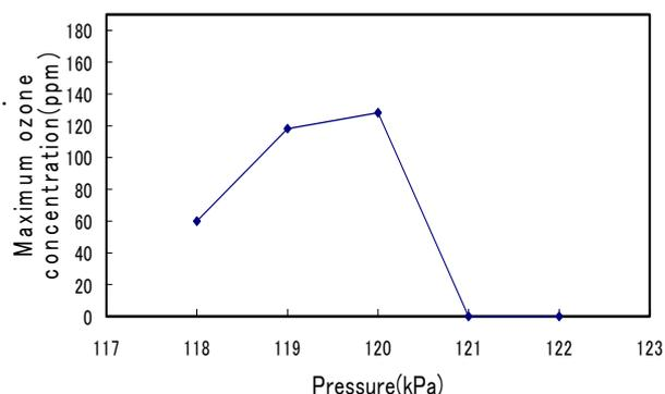
Fig. 11 Variation in maximum ozone concentration at the applied voltage of 1.8 kV.
