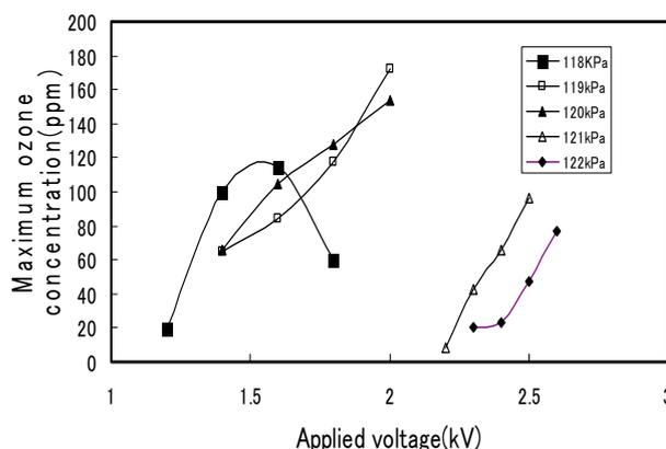
Fig. 12 Variations in ozone concentrations with various applied voltage and gas pressure.
