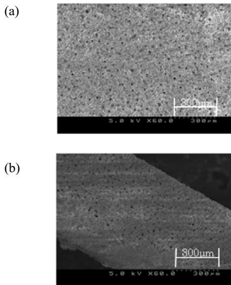
Fig. 2 SEM images of (a) the surface and (b) the cross section of SPG membrane.
