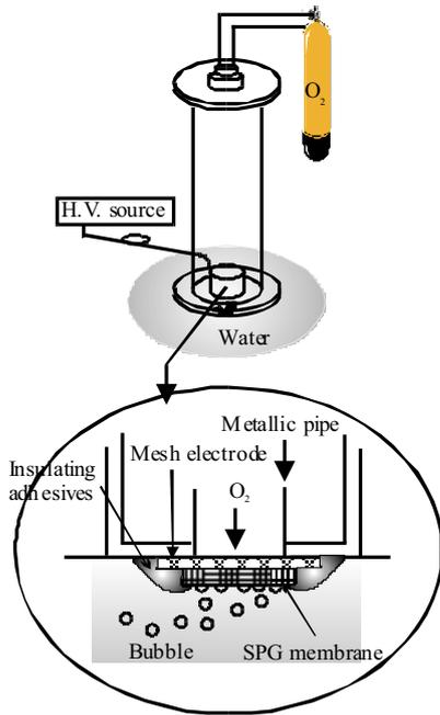
Fig. 1 Structure of proposed ozonizer.
