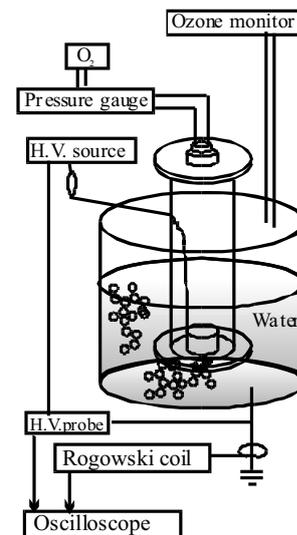
Fig. 3 Schematic diagram of experimental equipment.
