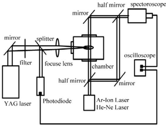
Fig. 1 Experimental arrangement.
