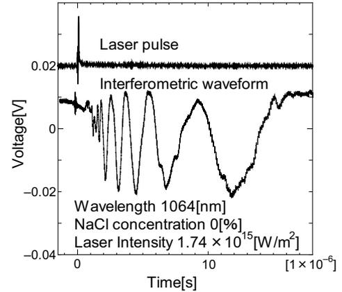
Fig. 2 Interferometric waveform and laser pulse.
