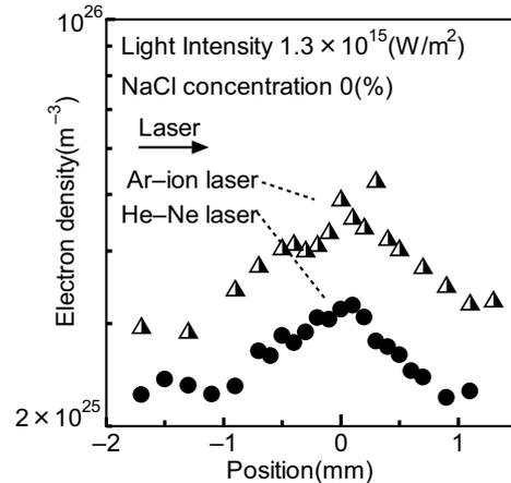
Fig.4, Comparison of electron density using Ar-ion laser and He-Ne laser.
