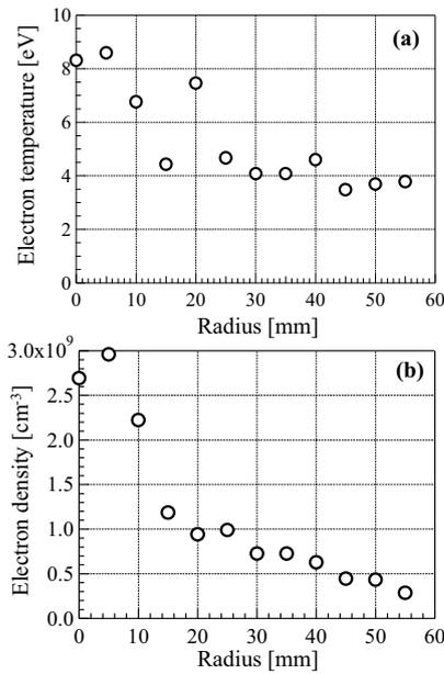
Fig.3. Radial distributions of plasma parameters of CCP. (a) electron temperature, (b) electron density.
