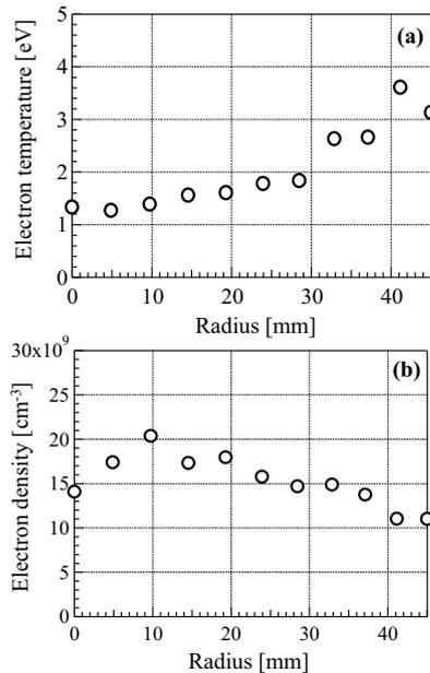
Fig.4. Radial distributions of plasma parameters of ICP. (a) electron temperature, (b) electron density.
