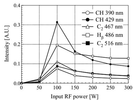
Fig.6. Intensity ratio of each line spectrum normalized to H<sub>α</sub> as a function of input RF power.
