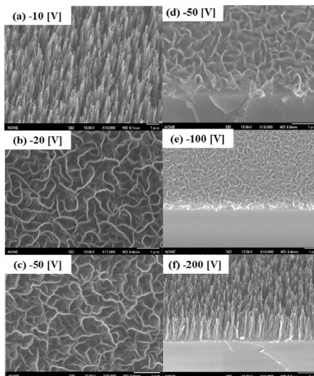
Fig.7. SEM images of carbon nanostructure by varying negative bias voltage using CCP and ICP. (a)-(c) CCP discharges, (d)-(f) ICP discharges.
