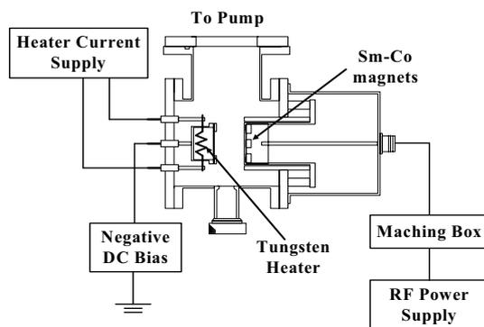
Fig.1. Schematic diagram of experimental apparatus of CCP.
