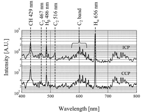
Fig.5. Optical emission spectra of methane and hydrogen plasma by CCP and ICP discharge.
