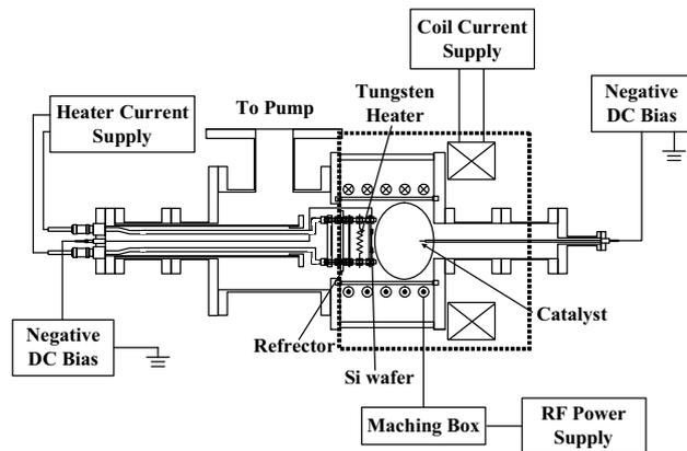
Fig.2. Schematic diagram of experimental apparatus of ICP.
