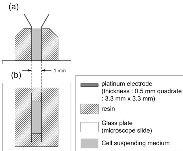
Fig.1 Schematic of the cross sectional (a) side and (b) top views of the application vessel..
