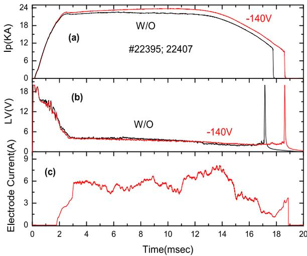
**Fig1:** Temporal evolution of (a)  $I_p$ , (b) Loop voltage for plasma discharges for with & without bias and (c) electrode current
