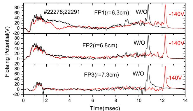
**Fig 3:** Temporal evolution of Floating potential in plasma discharge with (arrow position) & without bias.
