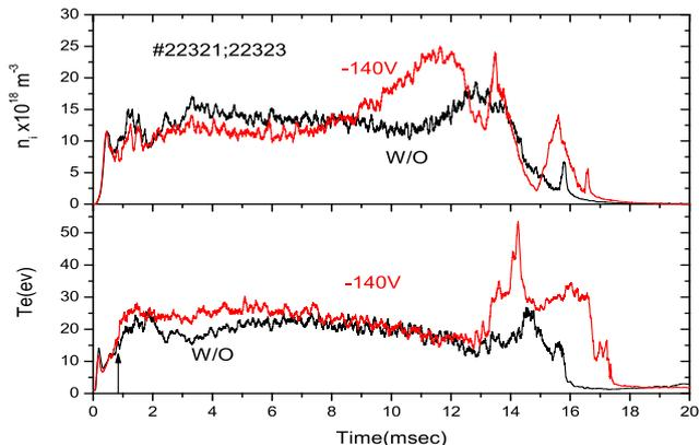
**Fig 5:** Temporal evolution of electron density and electron temperature of plasma discharges with (arrow position) and without bias.
