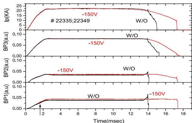
**Fig4:** Temporal variation of  $B_p$  with plasma discharge in three radial locations with (arrow position) and without bias. Top curve shows plasma current.
