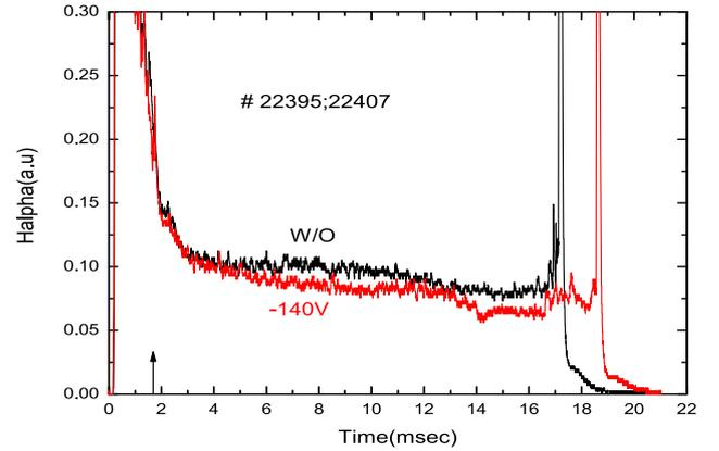
**Fig 2:** Temporal evolution of  $H_\alpha$ -emission for plasma discharges with (arrow position) & without bias voltage.
