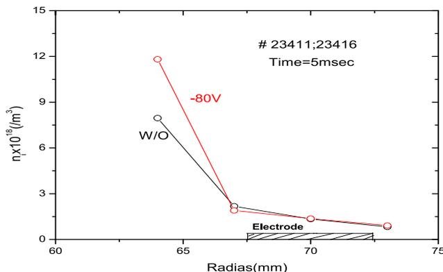
**Fig 6:** Spatial profile of the plasma density with and without bias up to 12 millimeter inside from the plasma edge.
