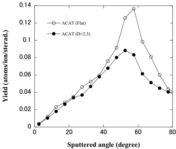
Fig. 6 Distributions of sputtered atoms calculated by the flat and the fractal ACAT under 1 keV  $H^+$  ions bombardment at an incident angle 80 degree from surface normal.
