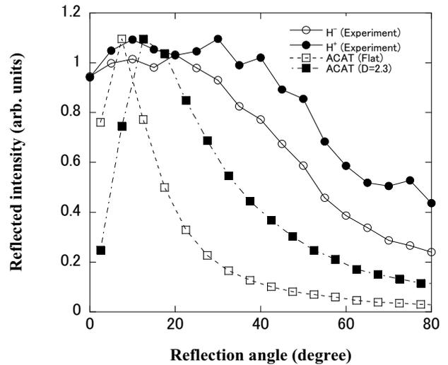
Fig.3 Measured reflected  $H^-$  and  $H^+$  intensities bombarded by 1 keV  $H^+$  ions at an incident angle 80 degree from surface normal. Also shown in the figure are the results calculated the flat and the fractal ACAT.
