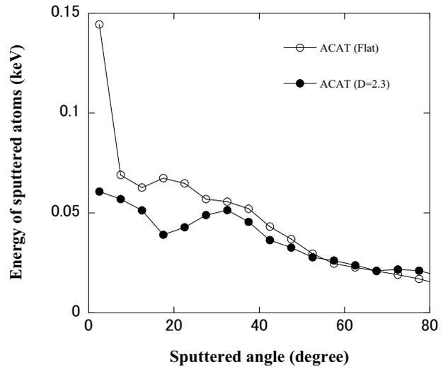
Fig. 7 Energies of sputtered atoms calculated by ACAT under 1 keV  $H^+$  ions bombardment at an incident angle 80 degree from surface normal.
