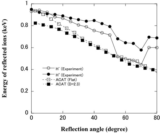
Fig. 5 Measured reflected  $H^-$  and  $H^+$  energy distributions bombarded by 1 keV  $H^+$  ions at an incident angle 80 degree from surface normal. Also shown in the figure are the results calculated the flat and the fractal ACAT.
