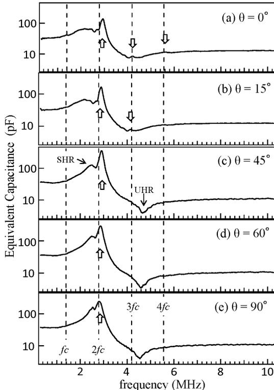
Fig.5 Variation of the probe equivalent capacitance depending on the angle between the cylindrical probe axis and the magnetic field. The electron cyclotron frequency was  $f_c=1.40$  MHz. The plasma frequency was  $f_p=4.3-4.6$  MHz.
