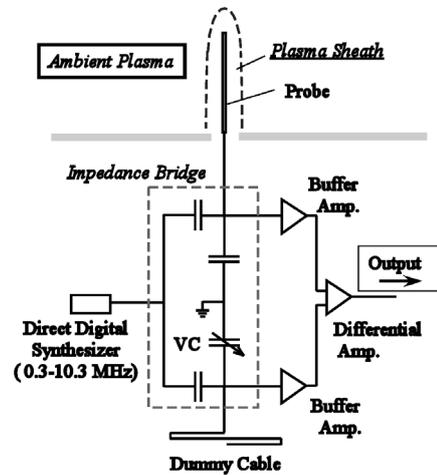
Fig.2 Block diagram of the impedance probe.
