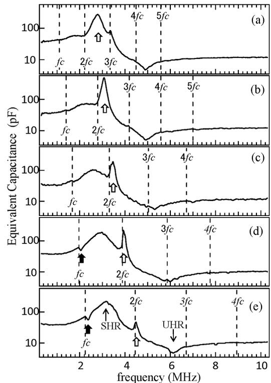
Fig.4 Variation of the probe equivalent capacitance depending on the magnetic field intensity. The cylinder probe was used. The magnetic field line was aligned along the probe axis. (a)  $f_c=1.12$  MHz, (b)  $f_c=1.40$  MHz, (c)  $f_c=1.68$  MHz, (d)  $f_c=1.96$  MHz, and (e)  $f_c=2.52$  MHz, respectively.
