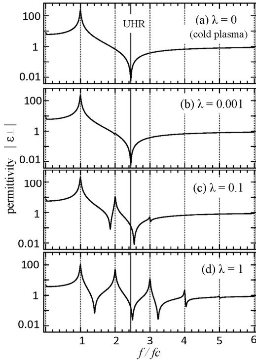
Fig.1 The perpendicular permittivity. (a) cold plasma case. (b)-(d) thermal plasma case. Characteristic frequencies are  $f_c=1.00$  MHz,  $f_p=2.24$  MHz, and  $f_v=0.01$  MHz.
