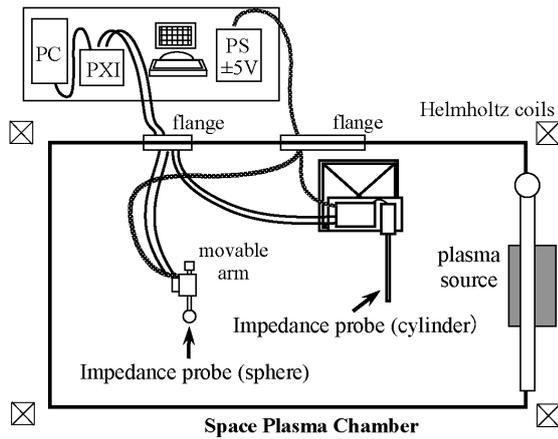
Fig.3 Configuration of the experiment. PS and PXI represent the  $\pm 5V$  power supply and the integrated instrument (signal generator and digital oscilloscope), respectively.
