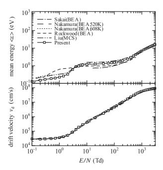
Fig. 5 Comparison between present results and other calculation values of mean energy and drift velocity.
