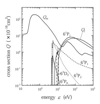
Fig. 1 Electron collision cross section of mercury. (to distinguish the cross sections, the line kind is indicated as for 6<sup>3</sup>P<sub>1</sub> (broken line), 6<sup>3</sup>P<sub>2</sub> (dotted line) and 6<sup>3</sup>D<sub>3</sub> (long broken line).)
