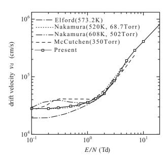
Fig. 4 Comparison between present result and experimental values of the drift velocity reported by other researchers.
