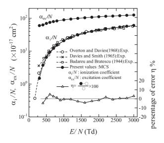
Fig. 6 Obtained ionization and excitation coefficients.
