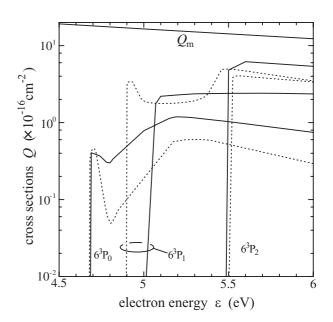
Fig. 2 Excitation collision cross sections (solid line : Hayashi, broken line : Hanne).
