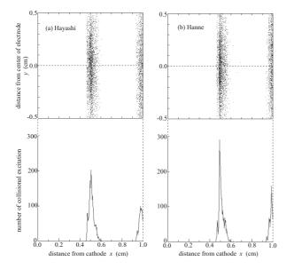
Fig. 3 Spatial distributions of excitation obtained by using cross sections shown in Fig. 2 ( $E/p_0 = 10$  V/cm  $\cdot$  Torr,  $p_0 = 1$  Torr).
