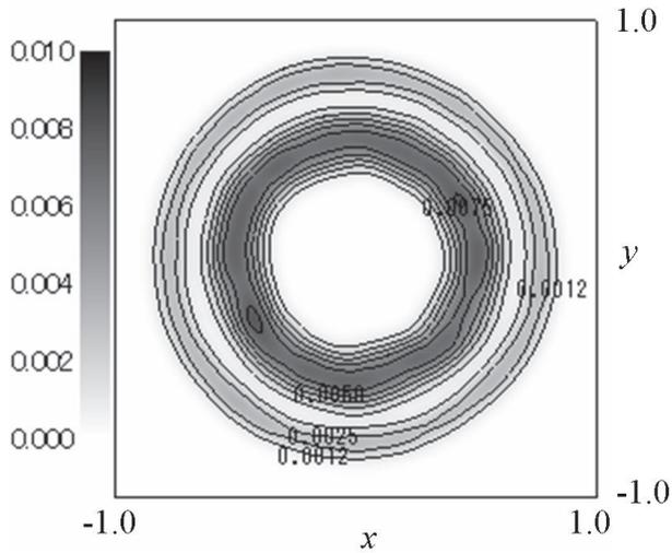
Fig. 6 The spatial profile of electron heat generation rate by the beam ions (i.e.,  $Q_{eb}$  in Eq. (8)) at  $t=5/\omega_{ci0}$ . Here,  $Q_{eb}$  is normalized by  $n_0 T_{i0} e B_{ex} / m_i$ , where  $n_0 = 5.0 \times 10^{19} \text{ m}^{-3}$  and  $T_{i0} = 100 \text{ eV}$ .
