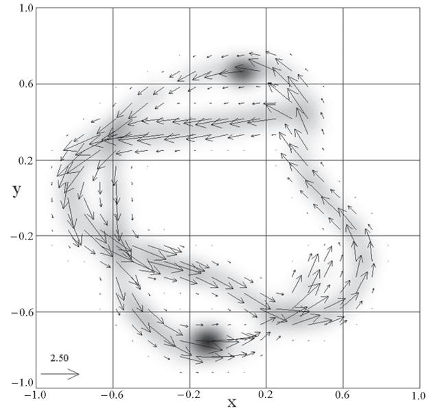
Fig. 2 Flow velocity profile of neutral beam injected fast hydrogen ions. Here,  $x$  and  $y$  are normalized by the wall radius. The beam flow velocity is normalized by the plasma ion thermal velocity  $\sqrt{2T_i/m_i}$ . The reference arrow is drawn in the left bottom corner, and its length corresponds to  $2.5 \sqrt{2T_i/m_i}$ .
