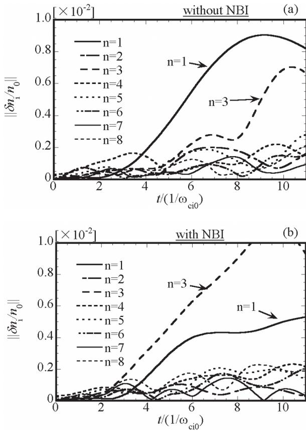
Fig. 5 Time evolution of the amplitude for several toroidal modes (from  $n=1$  to  $n=8$ ) of the ion density (a) for without NBI and (b) with NBI.
