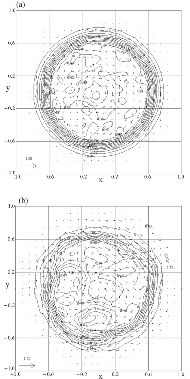
Fig. 4 Contours of electron pressure and electron flow velocity profile at (a)  $t=1/\omega_{ci0}$  and (b)  $t=10/\omega_{ci0}$  where  $\omega_{ci0} \equiv qB_{ex}/m_i$ . The reference arrow is drawn in the left bottom corner, and its length corresponds to the ion thermal speed  $\sqrt{2T_i/m_i}$ .
