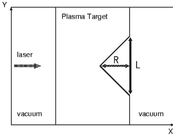
Fig. 1 Profile of a target containing a concave.
