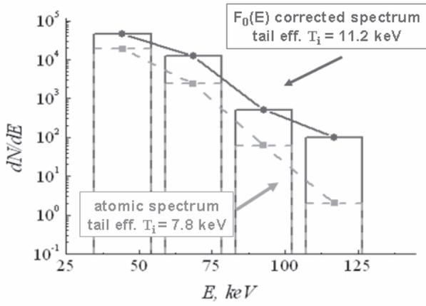
Fig. 3 Orthogonally measured PCX spectrum obtained by digital processing of natural diamond detector signals [3]. Target plasma  $R_{ax}=3.53$  m,  $\beta=0.20\%$ ,  $B=2.856$  T,  $n_e=1.5\times 10^{13}$  cm $^{-3}$ , tangential NBI heating (175 keV, 4 MW NBI#1, 150 keV, 1 MW NBI#2).
