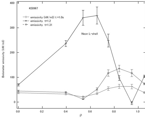
Fig. 5 Radial emission profile measured by bolometer.
