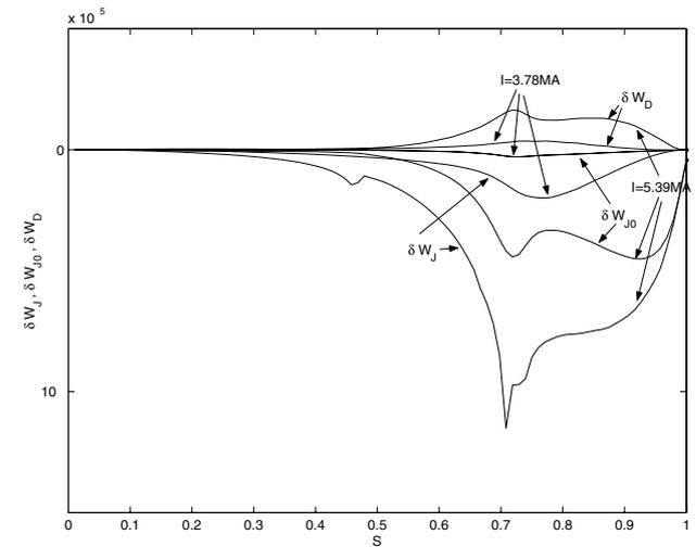
Fig. 4 The profiles of  $\delta W_D$ ,  $\delta W_J$  and  $\delta W_{J0}$  in a 2-period QAS stellarator reactor with toroidal currents of 3.78 MA and 5.39 MA. The curves shown from top to bottom correspond to 1) ( $\delta W_D$ , 5.39 MA), 2) ( $\delta W_D$ , 3.78 MA), 3) ( $\delta W_{J0}$ , 3.78 MA), 4) ( $\delta W_J$ , 3.78 MA), 5) ( $\delta W_{J0}$ , 5.39 MA) and 6) ( $\delta W_J$ , 5.39 MA), respectively.
