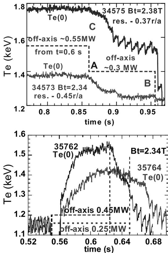
Fig. 1 (a) Variation of  $T_e(0)$  response with resonance position. (b) Same with ECRH power.
