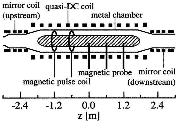
Fig. 1 Schematic drawing of the confinement region of the FIX device. The hatched region represents the translated FRC plasma.
