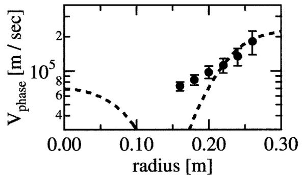
FIG. 6. Radial profile of the phase velocity of the excited wave in the  $z$  direction. The dashed line is the theoretical phase velocity of the shear Alfvén wave for the experimental condition.
