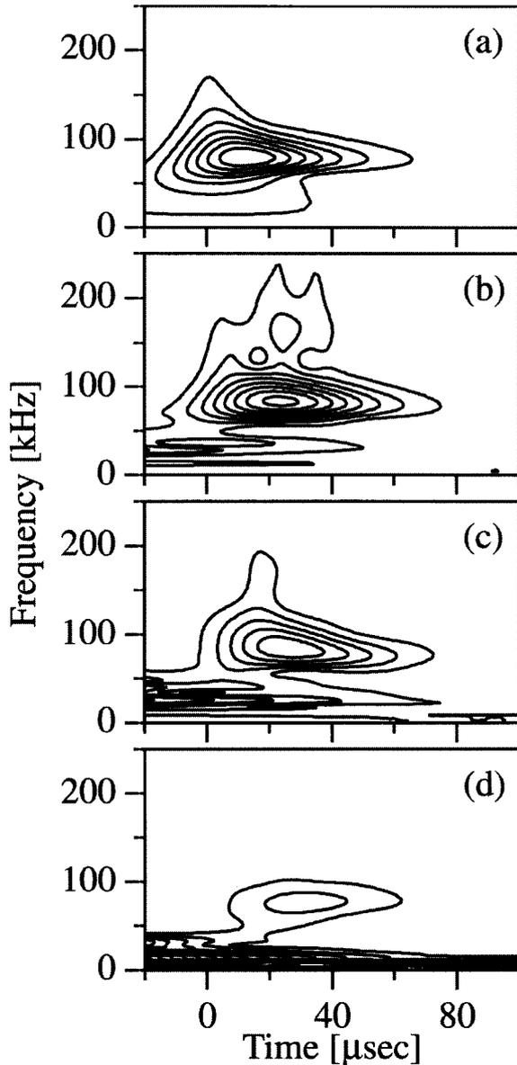
FIG. 4. The wavelet transform coefficients of the signals of (a) the coil current and three  $b_\theta$  probes at (b)  $z = 0.0$  m, (c)  $0.6$  m and (d)  $1.2$  m. The radial location of these  $b_\theta$  probes is  $r = 0.24$  m. In the figures (c) and (d), the contour scale is enhanced twice that in the figure (b). The magnetic pulse is started at  $t = 0$   $\mu\text{sec}$ .
