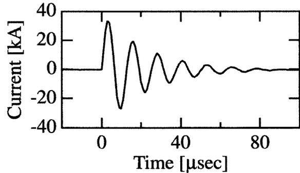
Fig. 2 The typical waveform of the coil current. The magnetic pulse is started at  $t = 0$   $\mu\text{sec}$ .
