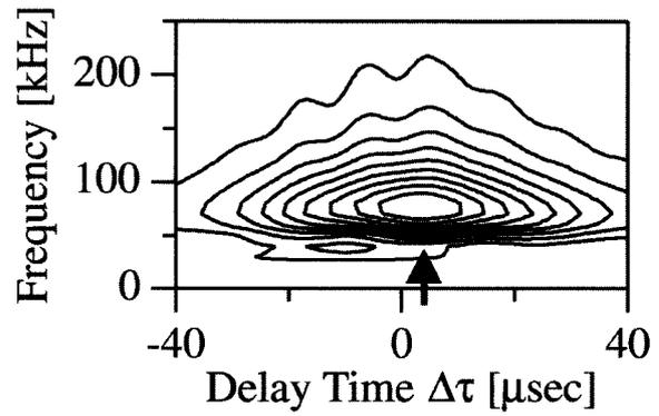
FIG. 5. The delayed wavelet cross-spectrum function for two  $b_\theta$  probe signals at  $z = 0.0$  and  $0.6$  m. The radial location of the  $b_\theta$  probes is  $r = 0.24$  m. The peak of the spectrum is shown by an arrow.
