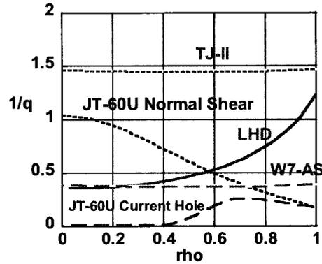
Fig. 2 Magnetic shear for tokamak and helical systems.
