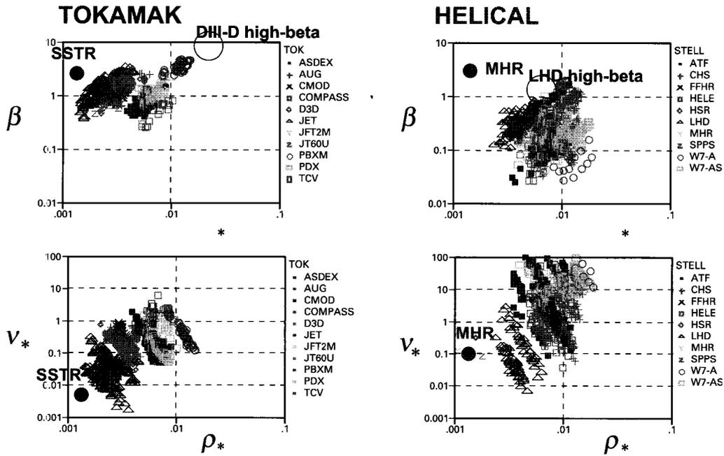
Fig. 1 Operational regimes and reactor requirements in tokamak and helical system.
