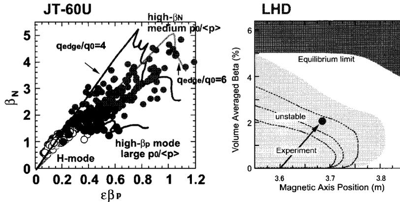
Fig. 5 Stability Limits in tokamak and helical systems.
