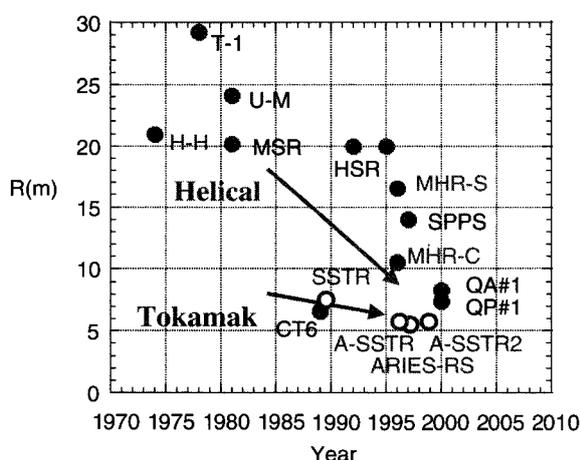
Fig. 7 Progress on reactor design for making compact and economical systems.
