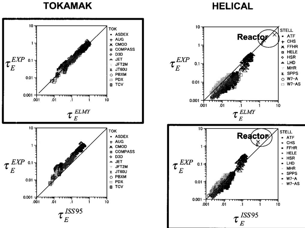
Fig. 4 Confinement scaling laws for tokamak and helical systems.
