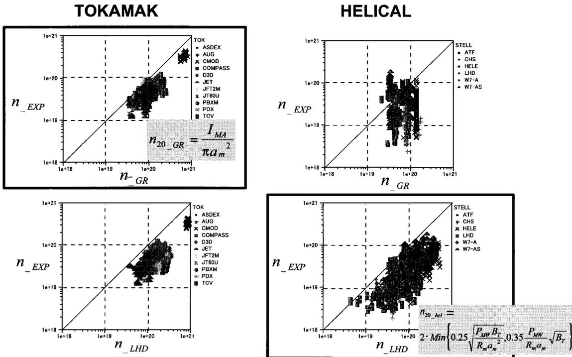
Fig. 6 Operational density regime of tokamak and helical systems.
