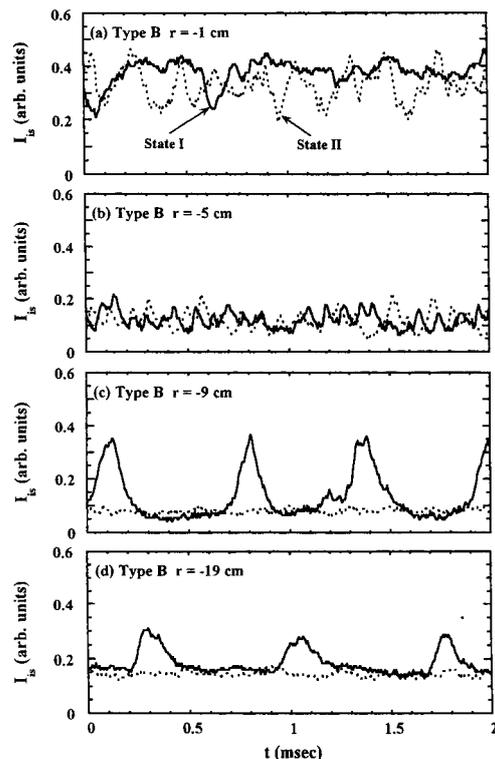
Fig. 4 Time evolution of ion saturation current  $I_{isr}$  ( $V_3 = 200$  V) for the radial location  $r$  of (a)  $-1$  cm, (b)  $-5$  cm, (c)  $-9$  cm and (d)  $-19$  cm (Eight individual traces have different shots).
