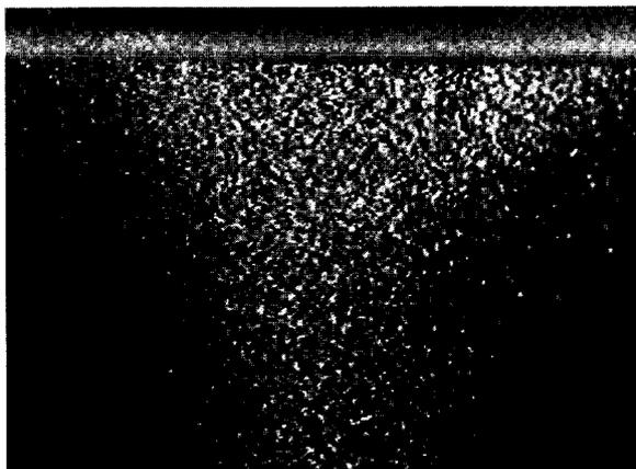
Fig. 6 Conical structure of a plasma suspended particle cloud.
