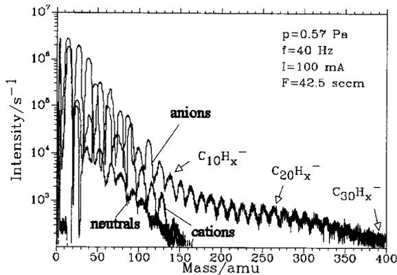
Fig. 5 Mass spectra with low resolution of positive and negative plasma ions and of neutrals from a DC glow discharge in methane.
