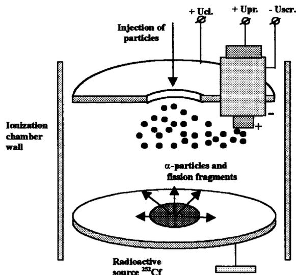
Fig. 7 Schematics of the electrode arrangement for particle removal from a dusty plasma.
