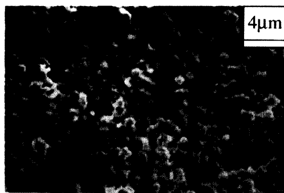
Fig. 3 SEM photograph of tungsten surface after the helium plasma irradiation at 1470 K for an incident fluence of (a) \sim 1.5 \times 10^{26} \text{ m}^{-2} .
