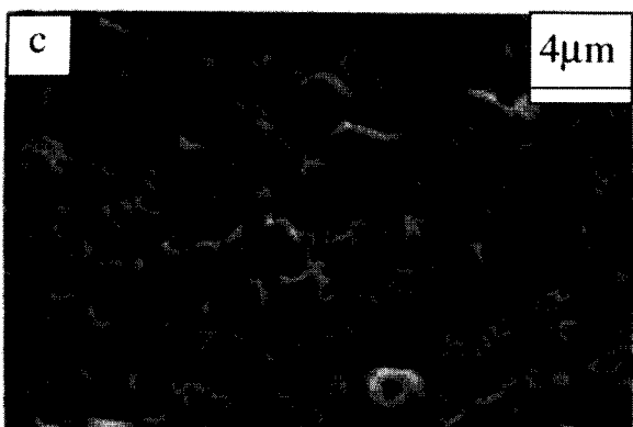
Fig. 2 SEM photographs of tungsten surfaces after the helium plasma irradiation at 1770 K for an incident fluence of (a) \sim 2.7 \times 10^{25} \text{ m}^{-2} ; (b) \sim 5.4 \times 10^{25} \text{ m}^{-2} and (c) \sim 1.1 \times 10^{26} \text{ m}^{-2} .
