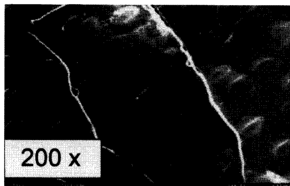
Fig. 3 A co-deposit on the toroidal limiter tiles. The layer structure reflects the topography of the graphite substrate.
