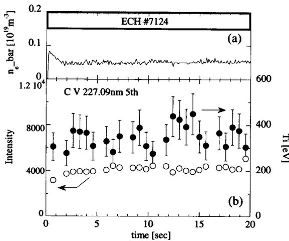
Fig. 4 (a) Time evolution of  $n_e$ , (b) Time evolution of  $T_i$  and line intensity on long-pulse ECH discharge.
