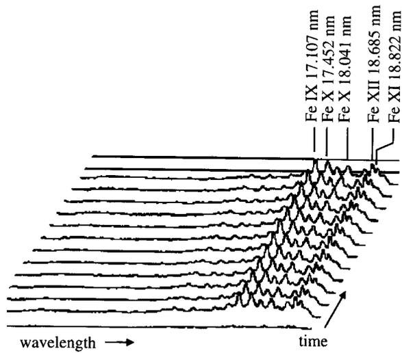
Fig. 3 Time-resolved display of spectra for 120 sec discharge in the 8-19 nm range with 133 g/mm grating. Exposure time for one frame is 10 sec. (#7132)
