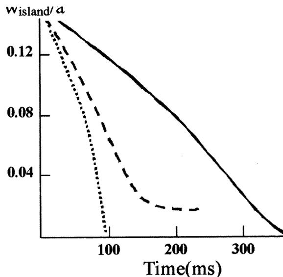
Fig. 5 CIEL2-2T: (3,2) mode island width normalized to minor radius vs time. Stabilization by ECCD (—) 0.9 MW, (---) 2.5 MW, (...) 2.5 MW modulated.
