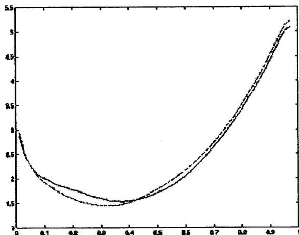
Fig. 4 CIEL2: safety factor profile vs  $r/a$ . (—) compound spectrum  $n_{\parallel} = 2$  &  $n_{\perp} = 2.9$ , (---) compound spectrum  $n_{\parallel} = 2.3$  &  $n_{\perp} = 2.6$ .
