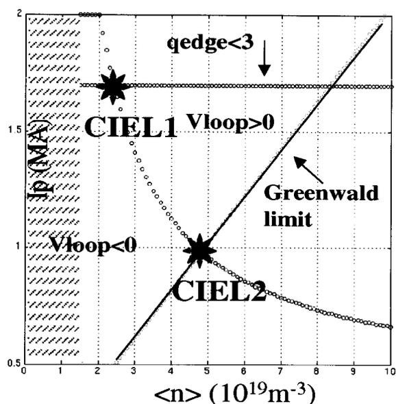
Fig. 1 Operating space at 3.8 T, 12 MW LHCD, 9 MW ICRH, 2 MW ECRH. The grey area refers to the ICRH coupling low density limit.
