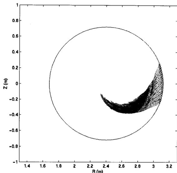
Fig. 2 CIEL1: example of LH rays propagation in the actual Tore Supra equilibrium. The launched spectrum is centred on  $n_{\parallel} = 2.6$  (60 rays).
