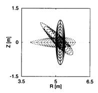
Fig. 2 Magnetic surface cross sections at  $\phi = 0$ ,  $(1/4)(2\pi/M)$  and  $(1/2)(2\pi/M)$  for an L=2 heliotron configuration (Conf. 2) with the partial quasihelical symmetry.
