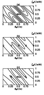
Fig. 4 The distribution of (a) magnetic field strength  $B_r$  (b)  $(1/B)(\partial B/\partial \theta_B)$  and (c)  $(\psi/B)(\partial B/\partial \psi)$  on r/a = 0.75 magnetic surface (one period) for Conf. 1 (Fig. 4.1) and Conf. 2 (Fig. 4.2).
