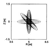
Fig. 1 Magnetic surface cross sections at  $\phi = 0$ ,  $(1/4)(2\pi/M)$  and  $(1/2)(2\pi/M)$  for a simple L = 2 heliotron configuration (Conf. 1).
