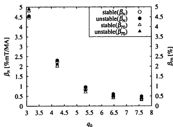
Fig. 2 Dependence of beta limit on  $q_0$  for the  $q$  profiles shown in Fig. 1. Here circular cross-section tokamak with  $A = 3$  is assumed.
