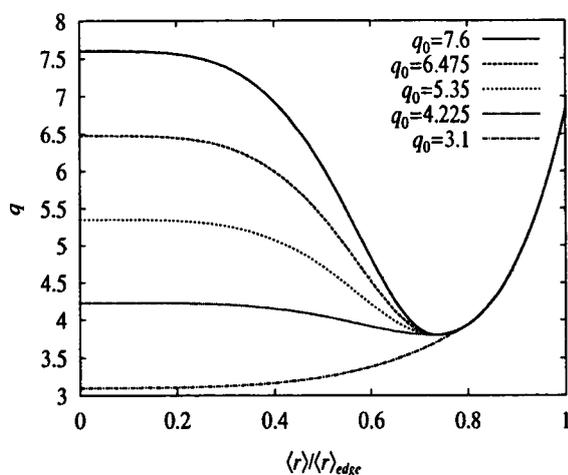
Fig. 1  $q$  profiles for reversed shear configurations as functions of normalized minor radius. Here  $q_{\text{min}} = 3.8$  and  $q_{\text{edge}} = 6.0$  are fixed and  $q_0$  is changed.
