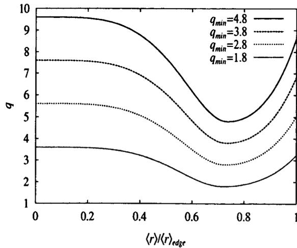
Fig. 4  $q$  profiles with various  $q_{min}$  as functions of normalized minor radius. Here  $q_0/q_{min} = 2.0$  and  $q_{edge}/q_{min} = 1.8$  are fixed and  $q_{min}$  is changed.
