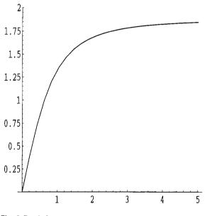
Fig. 2 Real frequency  $\omega$ , normalized to  $\omega_{e}$ , versus wavenumber k, normalized to  $k_{De}$ , when  $q_{d0}/e = -$ 1738.
