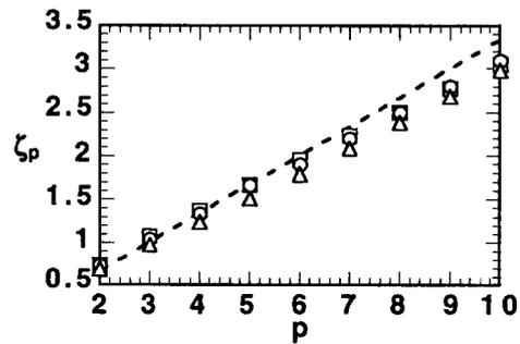
Fig. 4 Scaling exponent for the structure function versus order.
