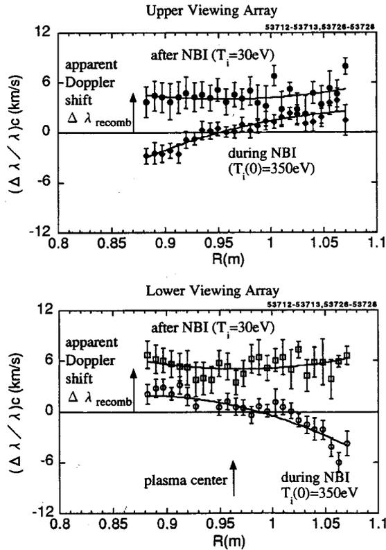
Fig. 4 The wave length shifts in the NBI heated phase and the after-glow recombining phase (CVI;  $\Delta n=7-6$ ,  $\lambda=343.5$  nm).
