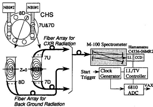
Fig. 1 The schematic of the optical system and the experimental arrangement. This system uses two fiber arrays viewing the beam from port 7D and 7U simultaneously, and one more fiber array to measure the background radiation at port 8D.
