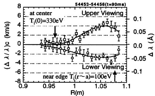
Fig. 3 The wavelength shifts measurement result given by single Gaussian fitting at the upper and lower viewing chords (CVI;  $\Delta n=8-7$ ,  $\lambda=529.2$  nm).
