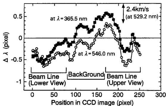
Fig. 2 The dependence of wavelength shifts  $\Delta\lambda$  on the position in vertical direction of the diffraction pattern (CCD image). Marks  $\circ$  and  $\blacksquare$  indicate fiber channels.
