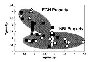
Fig. 2 The electron temperature-peaking parameter versus the electron density-peaking parameter (open triangle: ECH, open circle: NBI, solid rectangular: ECH overlapped NBI). The peaked T<sub>e</sub> and peaked n<sub>e</sub> profiles can not be achieved simultaneously.
