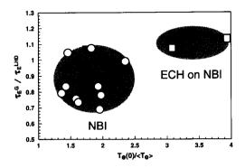
Fig. 4 The relation between the global confinement and the electron temperature-peaking parameter (open circle: NBI, solid rectangular: ECH overlapped NBI, open rectangular: ECH overlapped NBI in the low density region). The plots of global confinement of the combined heating plasmas in the low density region are located in the different region from the NBI data.
