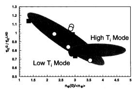
Fig. 3 The relation of the global confinement and the density-peaking parameter (open circle: NBI, solid rectangular: ECH overlapped NBI, solid circle: high  $T_i$ mode NBI). For low  $T_i$  mode plasmas, the global confinement decreases as the density-peaking parameter increases. The tendency for the high  $T_i$ mode plasma is different.
