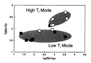
Fig. 1 The ion temperature-peaking parameter versus the electron density-peaking parameter (open circle: NBI, solid rectangular: ECH overlapped NBI). High  $T_i$  mode region and low  $T_i$  mode region are separated.
