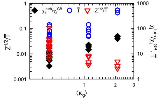
FIG. 1 Geodesic curvature dependence of zonal flow effect
