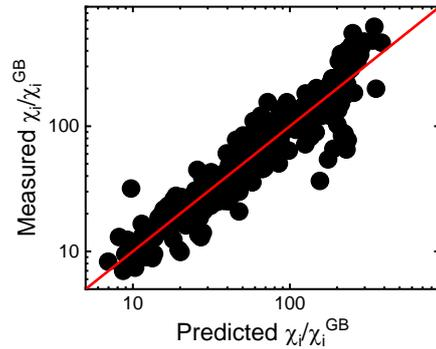
FIG. 2 Measured heat transport coefficient as a function of predicted heat transport coefficient.
