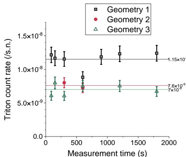
Fig. 1 Triton count rate per source neutron (s.n.) measured by the single crystal CVD diamond detector with a <sup>6</sup>LiF converter.
