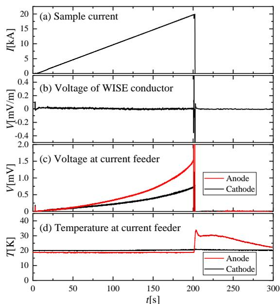
Fig.3 Time evolution of (a) sample current, (b) voltage of WISE conductor, (c) voltage at current feeder, and (d) temperature at the current feeder. The current feeder on the anode side has been burnout.
