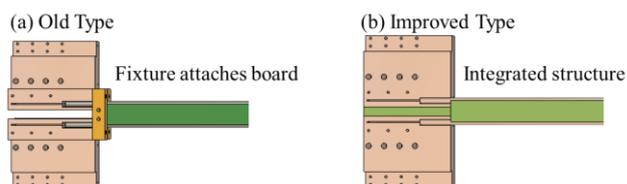
Fig.2 Previous WISE conductor (a) and developed WISE conductor (b). The WISE conductor is firmly anchored to the current leads.
