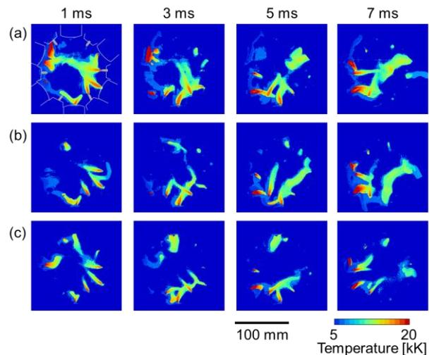
Fig. 4 High-speed visualized temperature distributions of diode-rectified multiphase AC arc at different arc currents; (a) 200 A, (b) 150 A, and (c) 120 A.
