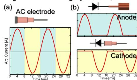
Fig. 1 Representative waveform of arc current for (a) MPA and (b) DRMPA.
