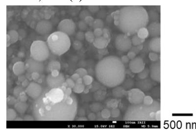
Fig. 5 Representative SEM image of the synthesized Si nanoparticles by multiphase AC arc.
