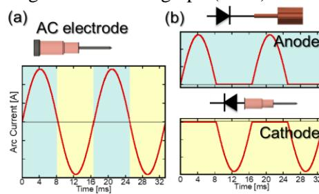
Fig. 1 Representative waveform of arc current for (a) MPA and (b) DRMPA.
