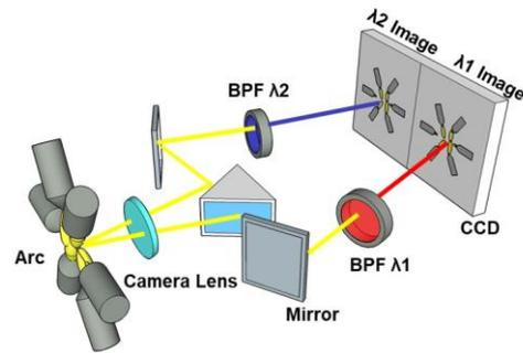
Fig. 3 Schematic image of visualization system with high-speed camera and band-pass filters.
