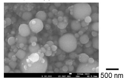
Fig. 5 Representative SEM image of the synthesized Si nanoparticles by multiphase AC arc.
