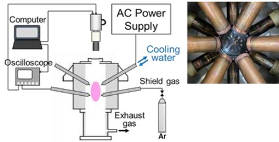
Fig. 2 Schematic diagram of the multiphase AC generator and measurement system arc.
