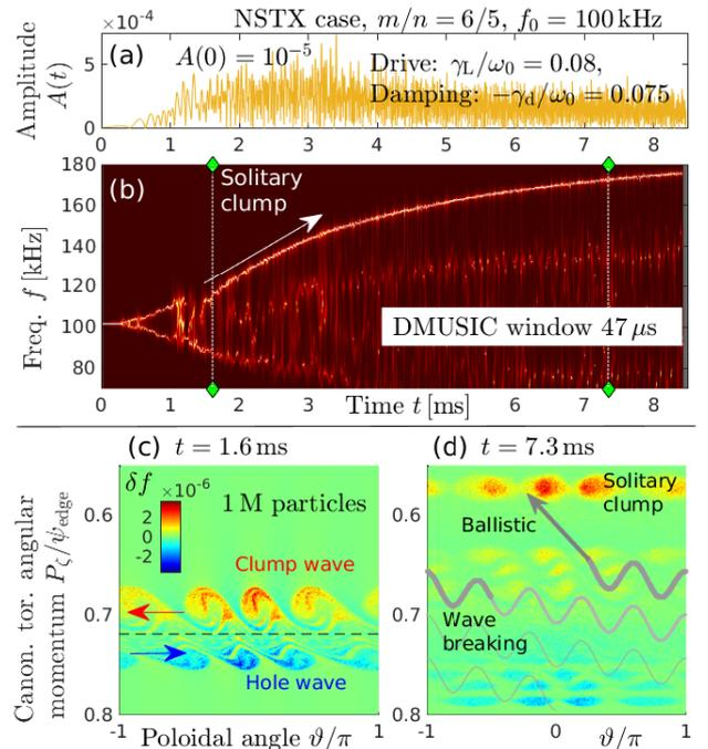
Fig. 1: DMUSIC spectrogram & snapshots of propagating phase space modes (a.k.a. holes & clumps).
