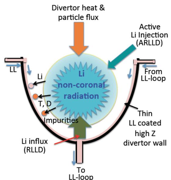
Fig. 1. A simplified schematic of RLLD/ARLLD low collisionality radiative divertor concept.
