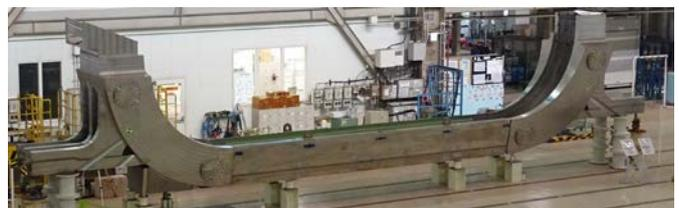
Fig. 3 Inboard sub-assembly during welding among basic segments.
