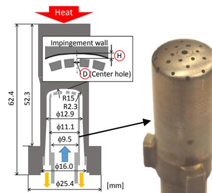
Fig 1. Cross-sectional view and inner cartridge of HEMJ test section
