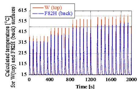
Fig. 4. Calculated temperatures for a thermal contact conduction per unit area between the F82H and Cu washer of  $4,000 \text{ W/m}^2\text{K}$
