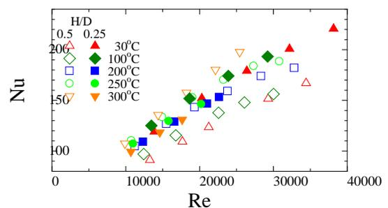
Fig 2. Effect of non-dimensional gap width on heat transfer performance of HEMJ
