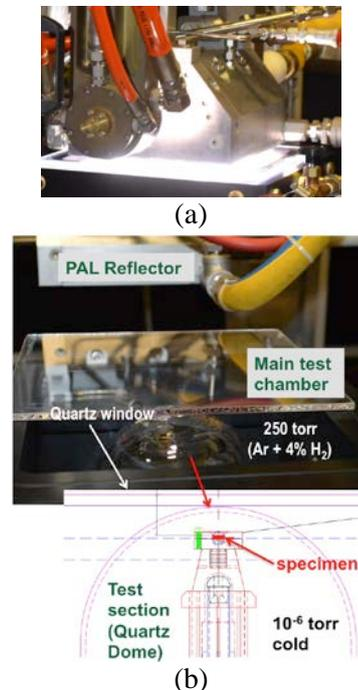
Fig. 3. Main components of the PAL HHFT: (a) PAL reflector focusing the energy onto the test chamber, (b) setup of main test chamber and specimen
