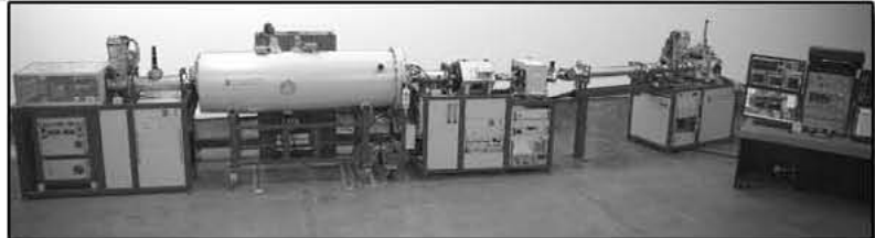
Pelletron Model 3SDH equipped with the NEC RF Charge Exchange Ion Source for H^+ and He^+ production and the Model RC43 analysis endstation
