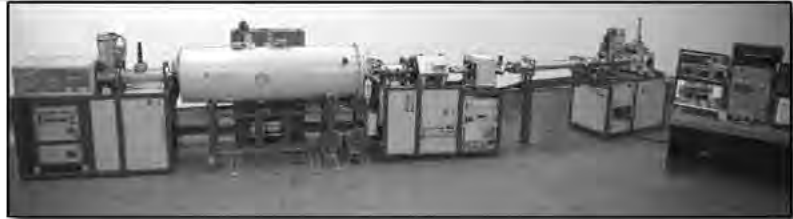
Pelletron Model 3SDII equipped with the NEC RF Charge Exchange Ion Source for H^+ and He^+ production and the Model RC43 analysis endstation
