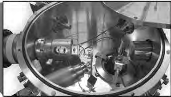
The interior of the RC43 can be equipped with moveable detectors in addition to a fixed detector for RBS and an electrostatic quadrupole quadruplet lens for micro RBS.
