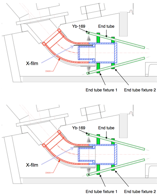
Fig.1. RT of welding part of the Feedthrough
