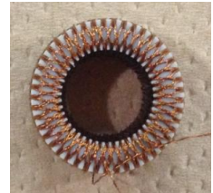
edge was observed about 150 [kA/m 2 ]. Fig.1 New Rogowski coil
