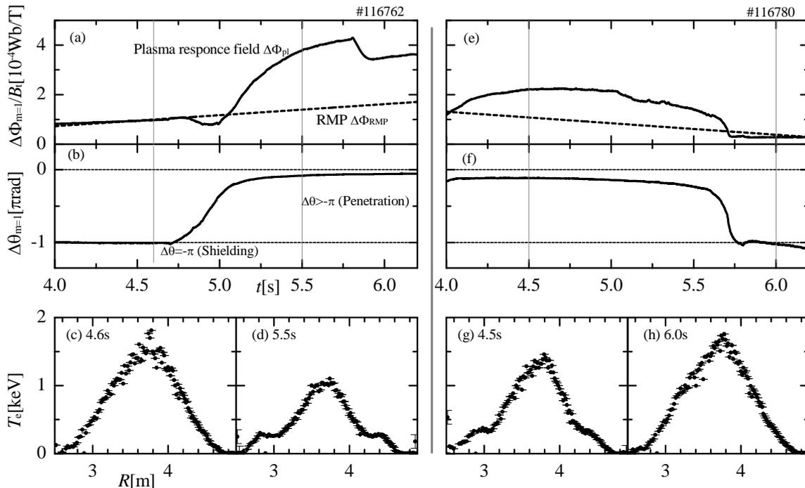
Fig.1 Time evolution of (a, e) Plasma response field (solid) and RMP (dashed), (b, f) phase shift  $\Delta\theta$ , (c, d, g, h) electron temperature. (Left) Case of RMP ramp up (Right) Case of RMP ramp down.
