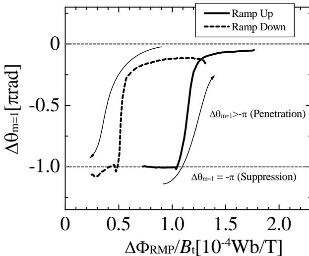
Fig.2 Relationship between phase shift and RMP. Solid and dashed lines indicate increasing and decreasing RMP cases respectively. Arrows mean time evolution.
