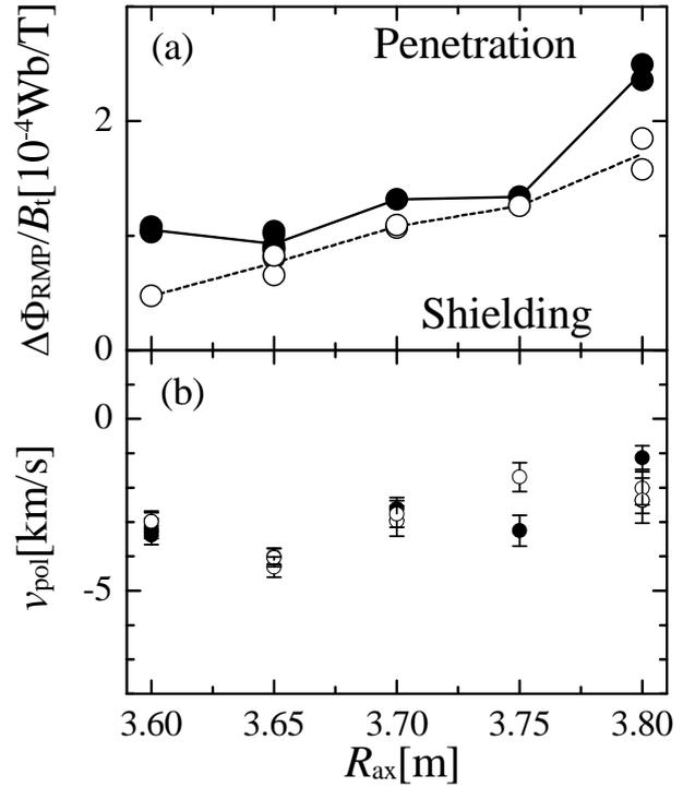
Fig.3 Magnetic axis  $R_{ax}$  dependence of (a) RMP threshold and (b) poloidal rotation. Closed and open circles indicate case of ramping-up and down respectively.
