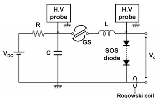
Fig. 1. The electric circuit of the high voltage pulse generator
