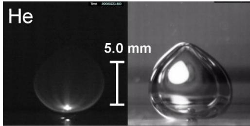
Fig. 3. A bubble and a discharge in the bubble.
