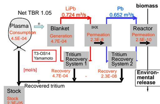
Fig.3 tritium flow in the biomass-fusion hybrid plant with LiPb blanket.
