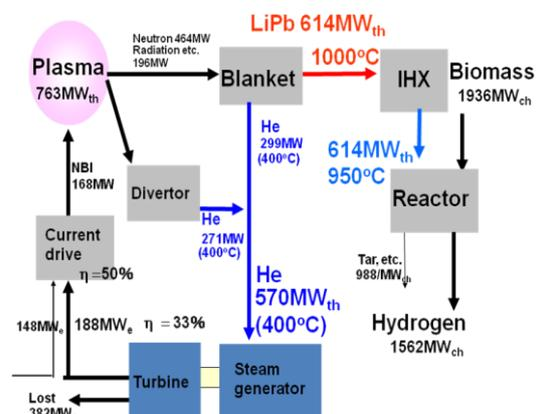
Fig.1 Energy balance of the fusion reactor for biomass fuel production.
