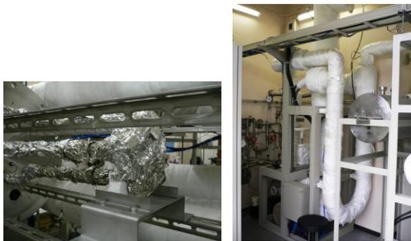
Fig.2 Lead Lithium loop in Kyoto university.
