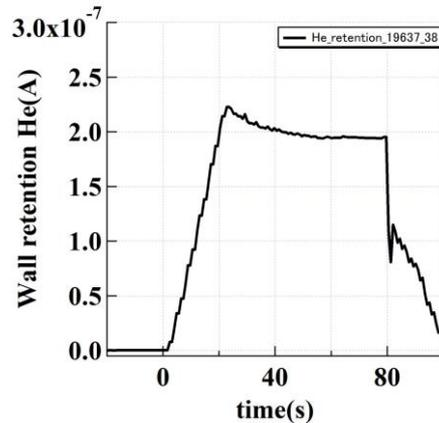
Fig. 3 Global gas balance for #19637(20s duration). The He puff was done during the pulse. All valves are closed.
