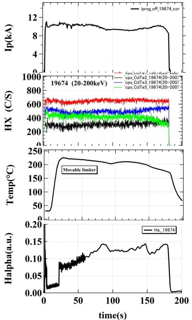
Fig.1 Time evolution of SST plasma; (a)  $I_p$ , (b) HX (co-red, vertical-blue, vertical-green, ctr-black), (c) temperature of the movable limiter, (d)  $H_\alpha$  from the CS region.
