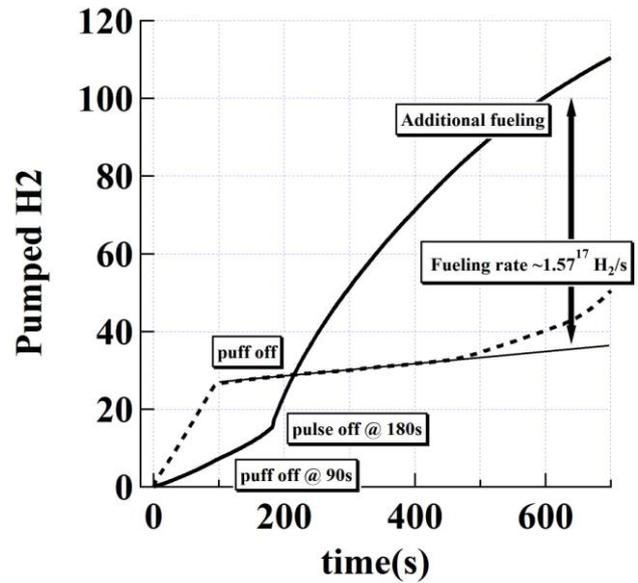
Fig. 2 Global gas balance for #19674(180s discharge). The puff was stopped at 90 sec.
