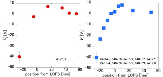
Fig. 2 Floating potential profile (a) obtained using the radial array probe in a single shot and (b) obtained in ten shots of plasma discharges
