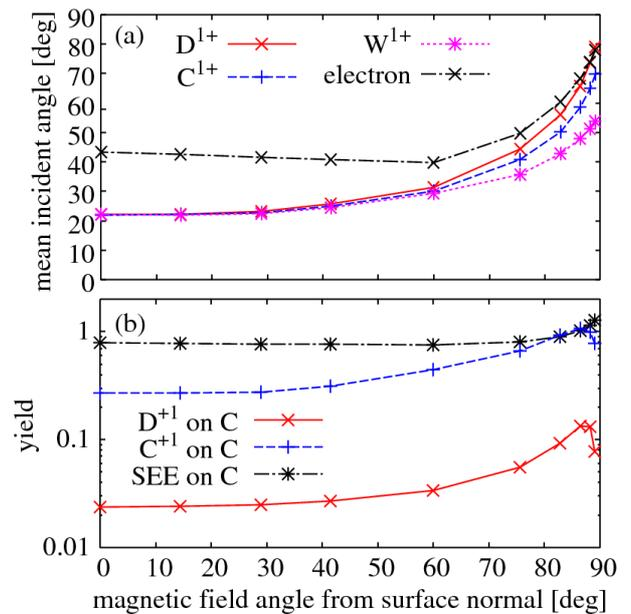
Fig. 1: (a) Incident angle distributions and (b) sputtering and secondary electron emission (SEE) yields obtained for various angles of the uniform magnetic field. The surface material is carbon.
